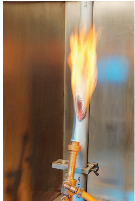
Carrying out a flame test according to the American standard UL 1581 at our Windsbach factory.
